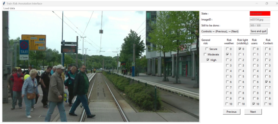
Figure 2: Risk annotation tools enabling to browse the Railsem19 dataset and to associate a risk level based on 5 criteria: general risk, weather, light, users and context according to 2 different scales.
