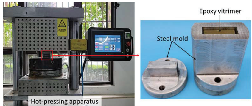
Figure 3. Experimental setup for welding.
