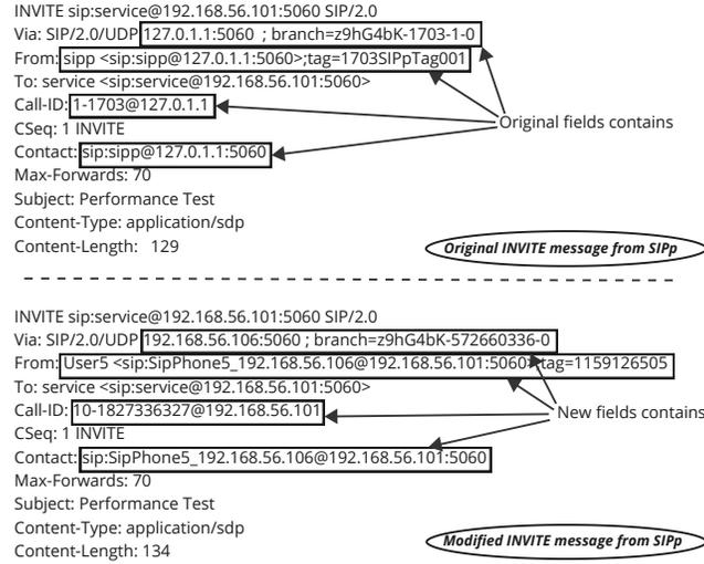
**Fig. 3.** Changes made to the content of INVITE message fields generated by SIPp to ensure the consistency of the generated data.
