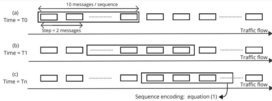
**Fig. 5.** Description of INVITE sequence detection approach: the sliding window size is fixed to 10 messages and the step forward to 2 messages per time unit. If the sequence contains at least 2 malicious messages, it is labeled as malicious. Otherwise, it is a legitimate sequence.
