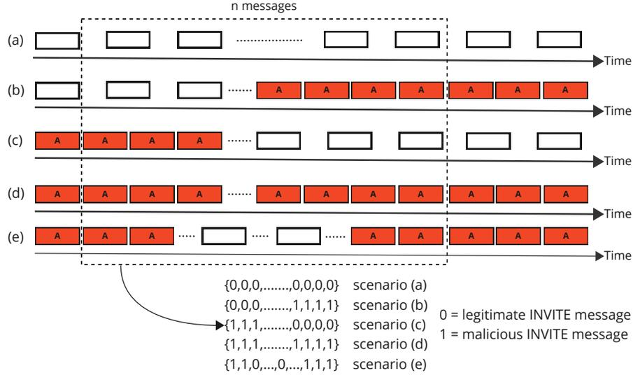
**Fig. 4.** The different generated sequence scenarios of INVITE traffic. (a) legitimate sequence, (b) a sequence that ends with malicious traffic, (c) a sequence that starts with malicious traffic, (d) a sequence containing nothing but malicious traffic, (e) a sequence containing legitimate traffic in the middle.
